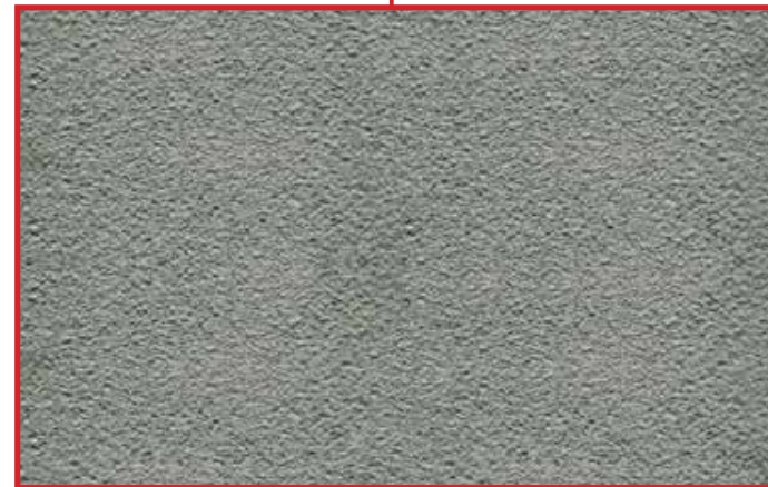
CONCRETE W/ EPOXY FINISH
